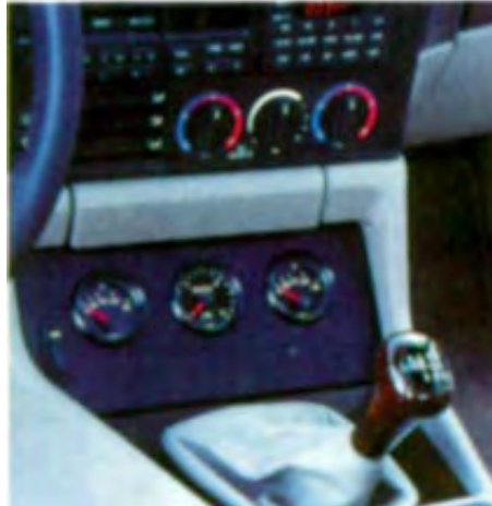
Along with the tidy supercharger installation, Dinan adds a row of gauges for boost pressure, engine-oil temp, and differential-oil temp.
