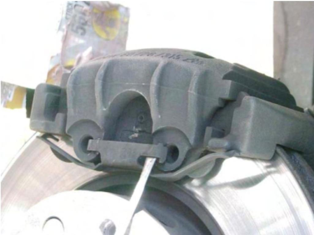
**4)** At this point, you should be able to wiggle the caliper off the bracket by pulling away from the rotor. Have a box or spare jack stand handy to rest the caliper on so you don't stress the hose.
