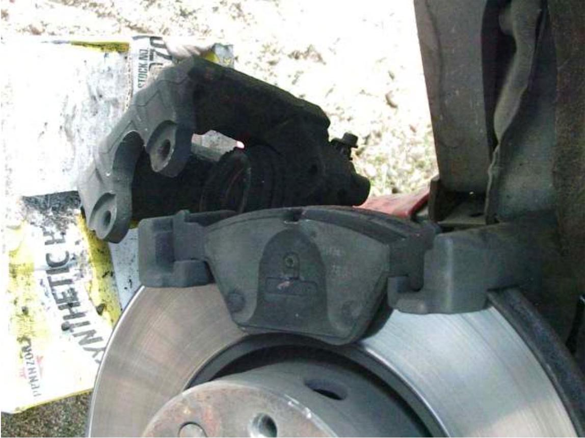
**6)** If you haven't done so already, hook up a bleeder hose and jar as described above, loosen the bleeder screw and push the piston in. This is easy when the fluid (old and dirty) can escape through the tube.
