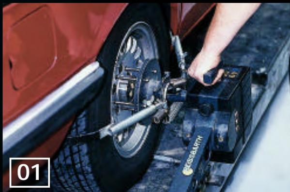
The first stage is to put the car on the ramp with its wheels on the circular discs and then to fit the four cameras. These will only fit BMW wheels with the five location holes. So if you have weird alloy wheels, you'll need to give prior notice so a set can be found and fitted for the operation. Tyre pressures need to be correct and if the car has been lowered or has a bodykit the special adapters to lower the cameras need to be fitted.
