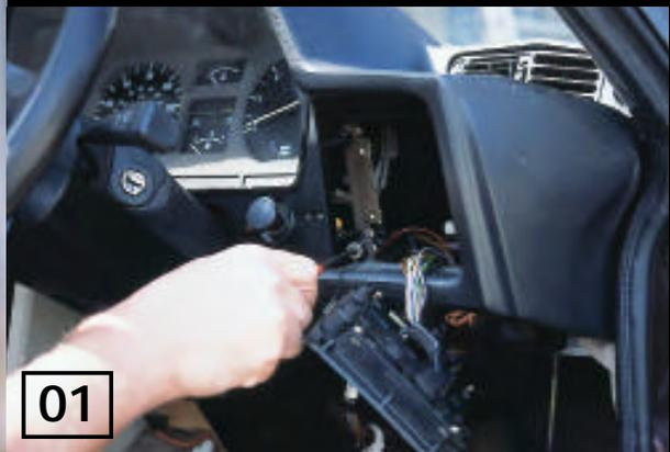
01 First job is getting the instrument pod out. We used a 1983 628CSi for this, which is one of the hardest to do. Remove the black plastic panel either side of the cluster, which comes out to reveal the lower two retaining screws.
